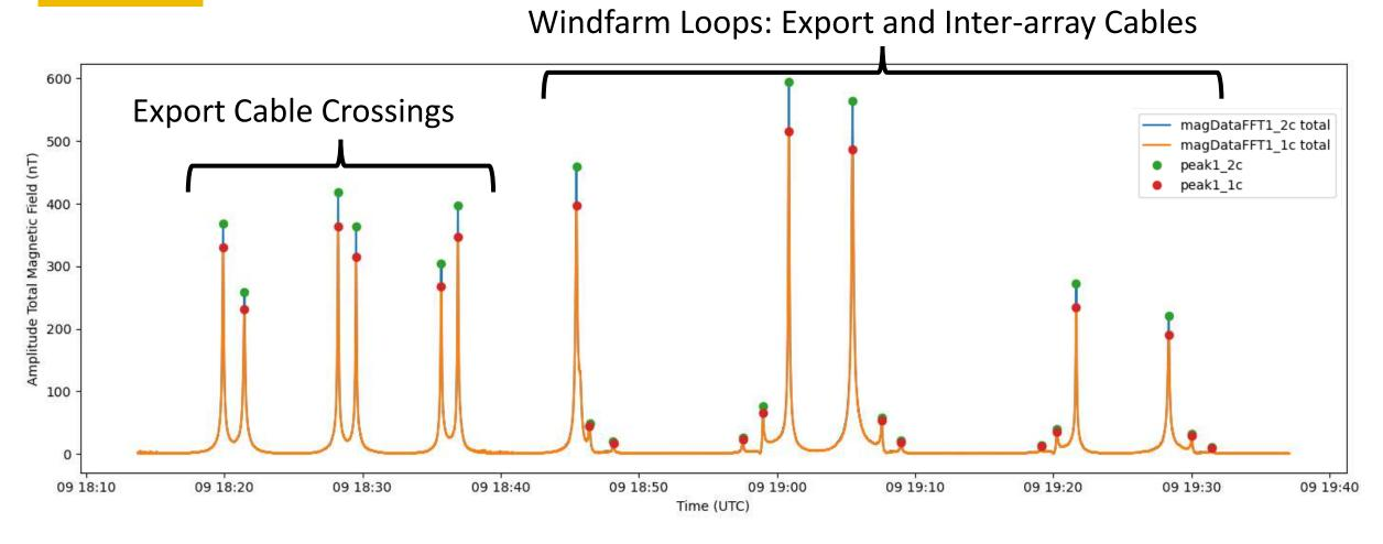
Example of the Total Magnetic Field Amplitudes and the peak picks for the Forward Port Top and Bottom Pair – these picks are used to determine Depth of Burial
